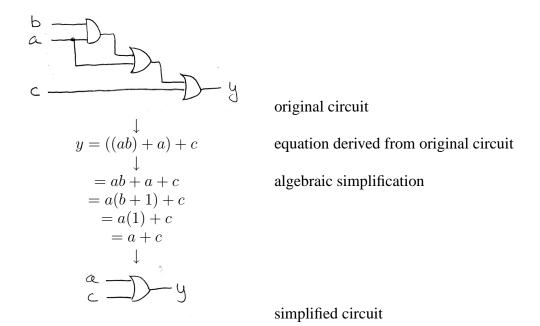
Another use for Boolean algebra is in circuit *verification*. Given a circuit and a Boolean equation, we can ask the question "do the two different representations represent the same function." The first step would be to derive a new Boolean expression based on the circuit. Then through algebraic manipulation we could manipulate the expressions until they match, thereby "proving" the eqivalence of the two.
