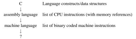
How are these instructions carried out? What happens to the machine instructions? One thing we can do is to read them into a simulator (such as SPIM). However, most of the time, we are interested in actually running the instruction on real hardware. How does the hardware execute our instructions? That is the topic of the remainder of the semester.
